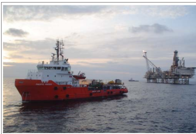
Figure 4. Dual-purpose cable operation and shooting vessel Pacific Raider during operations near central Azeri platform. The cable and gun systems are modularized for alternate back-deck deployment.
